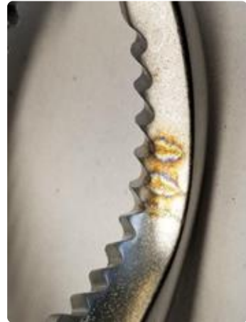
Bone clamp with fractures and staining
