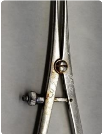
Staining on an eye caliper
